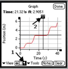
b. A little triangle will appear, connected to crossed lines. The mark can be moved around with the cursor, and the x and y values of the graph will show at the top.
