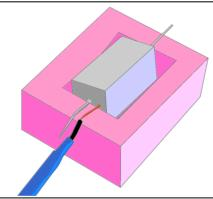
4. Close the heat cell in its insulating box by wrapping it with a rubber band and connecting the two clip leads to the metal wires that are sticking out.
