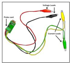
1. Connect the flexible cable from the VoltageCurrent probe to the VoltageCurrent probe card. Plug the VoltageCurrent probe card into Port A of the Interface Box. Be careful not to bend any of the copper prongs, or it won't work.
