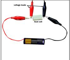
3. To measure the current in a wire, you have to break the wire and force the current to go through your current probe. The convention is that current is positive when it flows from a positive to a negative voltage, that is, from red to black. For the current through the probe to be positive, it should flow into the yellow clip lead and out of the green clip lead. Here is how to measure current going through a heat cell attached to a battery. Current is measured in amperes (A).
