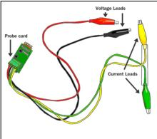
2. Voltage difference is measured in volts (V). The red clip lead goes to the positive (+) place, and the black clip lead goes to the negative (-) place. Here is how to measure voltage between two ends of a heat cell attached to a battery:
