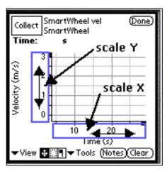
b. If you stretch or shrink the scale a great deal, it will switch by a factor of 1000, shown as 10^3 (for large numbers) or 10^-3 (for small numbers). For example, in the following screen, time is in milliseconds (1/1000 of a second) and light intensity is in kilolux (1000 lux).
