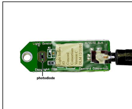
The Light Probe has a photodiode that responds mainly to visible light, which is also the light needed for photosynthesis by plants. It produces a voltage depending on the light level. There are two ranges, one that can measure bright sunlight, and the other for indoor light.
