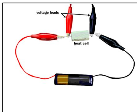
Current is the amount of electricity flowing, a bit like the current in a stream. Current can be pictured as the total number of electrons flowing per second through a wire or other substance. You can imagine measuring current by setting up a tollbooth in a wire and simply counting how many electrons went by each second. Current is measured in amperes (A).
