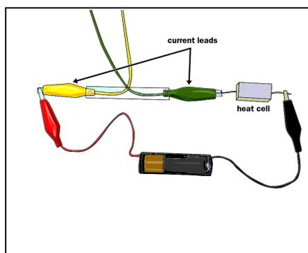
Electrical power, the rate of using energy, is the voltage difference times current. It can be pictured as the number of electrons flowing per second, multiplied by the energy each one loses ( $P=IV$ ). Power is measured in watts (W).
