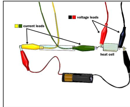
Electrical energy is the power accumulated over time. It can be pictured as the total number of electrons that flow, multiplied by the energy that each one gains (or loses). Energy is measured in joules (J). To measure the energy transferred into a heat cell from a battery, you must measure both voltage and current (see diagram above). The CCProeware will calculate and display the energy from these measurements.
