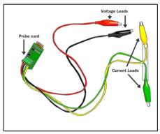
The Voltage/Current Probe measures either voltage or current. It can also measure both at the same time. The CCProbe software can use these readings to calculate and display power (watts) and energy (joules).
