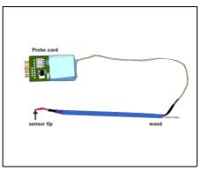
The only sensitive part is the tip where two special bare wires are twisted together. The wires produce a voltage depending on the temperature, and the CCProbe software converts this to degrees (C or F). The response is very fast, because the two wires are small and easily heated or cooled by whatever they touch.
