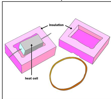
3. Insert the tip of the Temperature probe into the small hole in one end of the heat cell. Put on the insulation cover and close the box with a rubber band.
