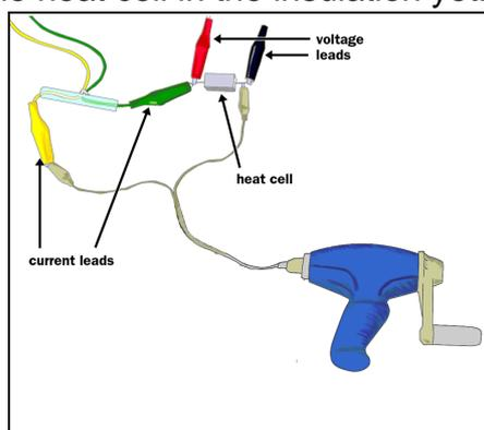
4. Start the software to record power. This measures the electrical power, in watts, that you are supplying to the heat cell with the Genecon.
