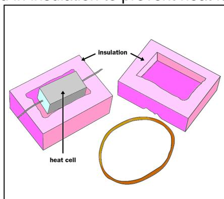
3. Remove the heat cell from its insulation. Attach the two leads of the Genecon to wires extending from the heat cell. Also connect the voltage leads and the current leads of VoltageCurrent probe to the heat cell. Follow the diagram carefully. Don't put the heat cell in the insulation yet.
