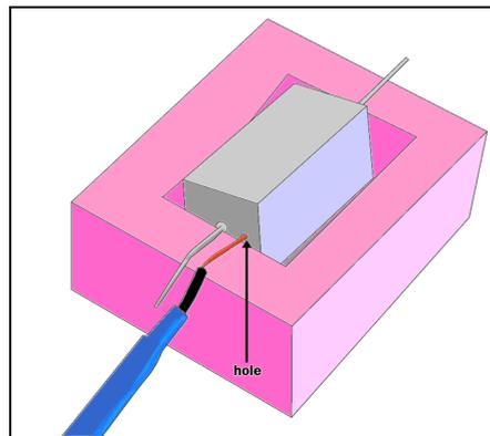
4. Use a 2-AA battery pack, which will supply somewhat less than 3 volts, to warm the heat cell. You can use the battery pack on the air cart for this. Attach one of the battery leads, but not the other, to the heat cell.
