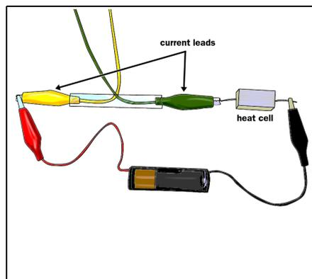
4. Electrical power, the rate of using energy, is voltage difference times current. It can be pictured as the number of electrons flowing per second, multiplied by the energy each one loses. Power is measured in watts (W).
