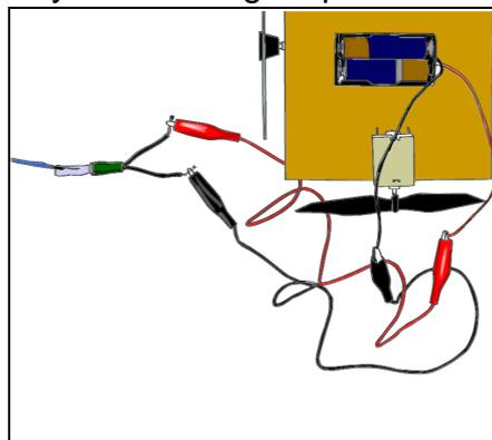
6. Monitor the temperature plot. Let it run for 30 seconds, then disconnect the second lead and let it run for another 30 seconds. Stop recording.
