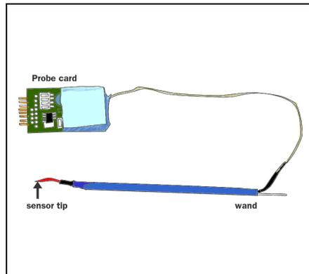
1. Connect the flexible cable from the Temperature probe to the Temperature probe card. Plug the Temperature probe card into Port A of the Interface Box. Be careful not to bend any of the copper prongs, or it won't work.
