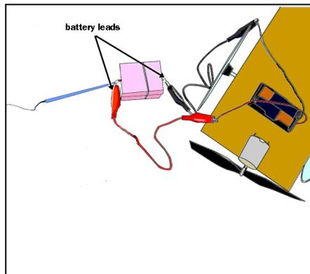
7. Heat the cell for 60 seconds, then disconnect one battery lead. Let the graph run another 60 seconds so that you can watch the cooling of the heat cell.
